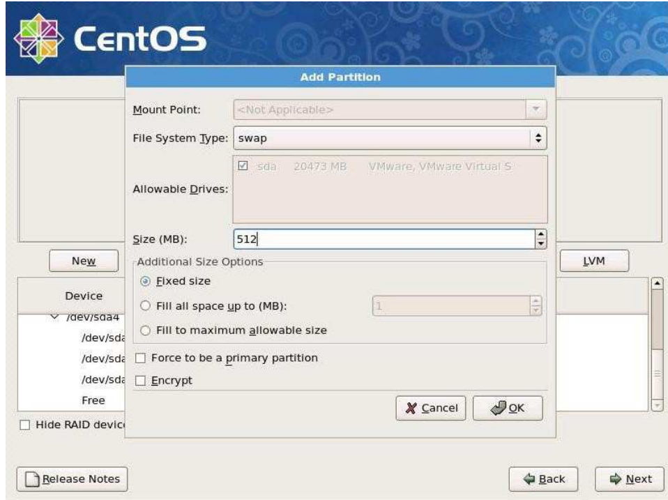
Figure 12 : Partitioning the Hard Disk – Swap Partition
