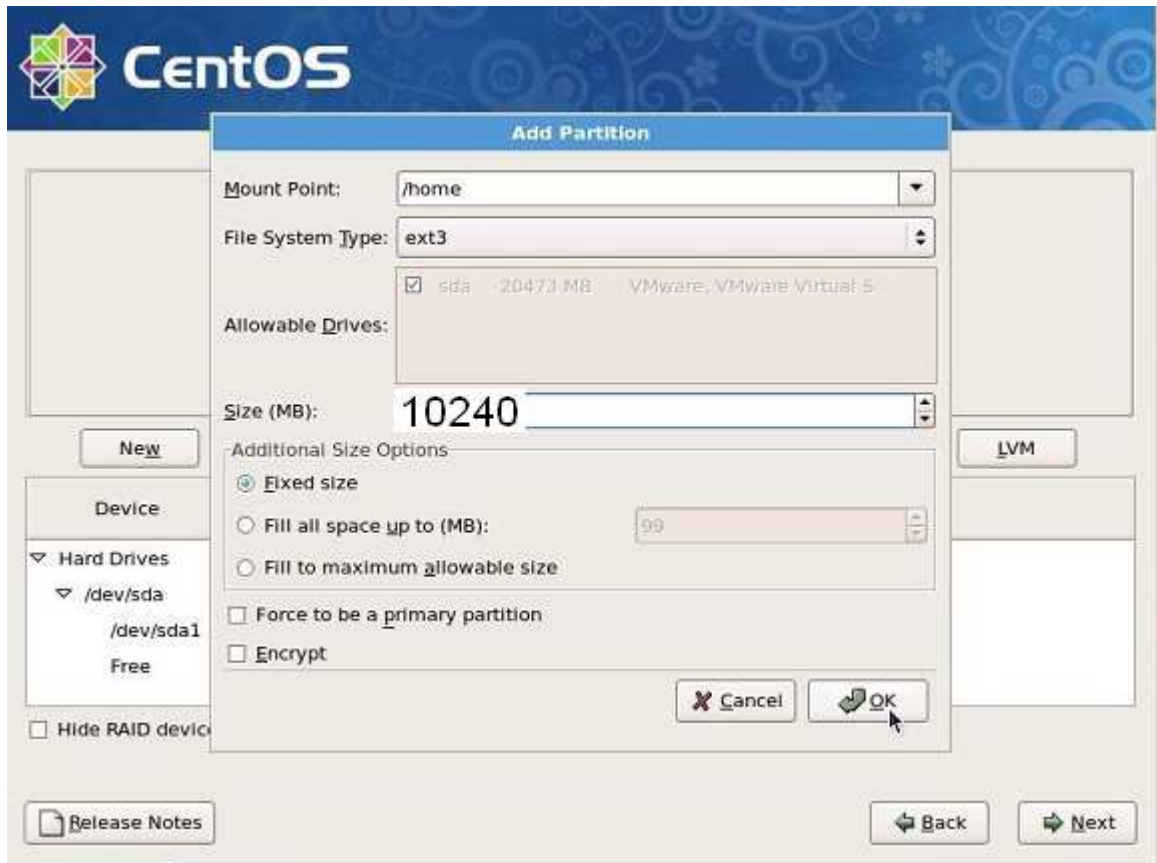
Figure 7: Partitioning the Hard Disk - /home
